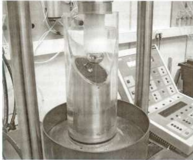
FIGURE 8.1 Femoral hip stem neck fatigue testing setup according to ASTM F2068 – 09 [15]. (Image courtesy of Biomet)
